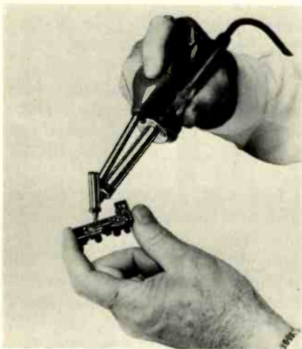
Fig. 3—Applying a desoldering iron to a simple soldered connection.
