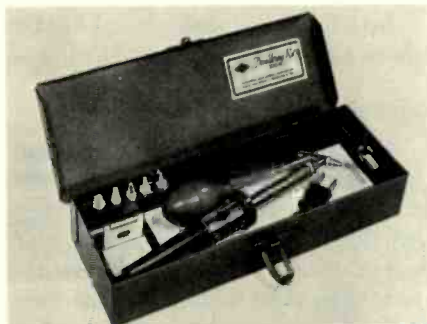
Fig. 1—A desoldering kit designed to quickly and safely remove solder from heretofore difficult, if not impossible problem situations.
