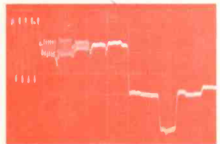
Fig. 7—Multiburst-horizontal, Fine tuner adjusted just past color threshold.
