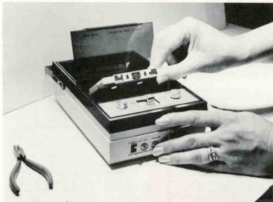
Fig. 1—Cassette tape recorder has pop-up feature for easy loading.
