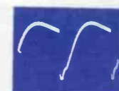
9 SR201 CATHODE JUNCTION 13V. P-P HORIZ. RATE
