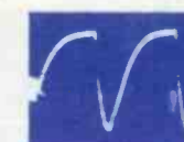
10 SR201 ANODE JUNCTION 16V. P-P HORIZ. RATE
