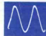
11 PW200-TP4 HORIZ. CONTROL PLATE 20V. P-P HORIZ. RATE
