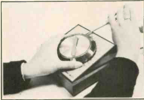
Fig. 7—Place control on non-slip surface. Turn knob until any snap leg is in position shown. Leg of snap shows as a dark, clear spot in the brown part of upper knob. There are 3 legs. Arrow points to one. Push hard against side of knob toward arrow, place flat screwdriver under edge close to leg and lift up about 1/2 in. Release hand pressure, move hand around, placing thumb under knob to hold knob up, remove screwdriver.
