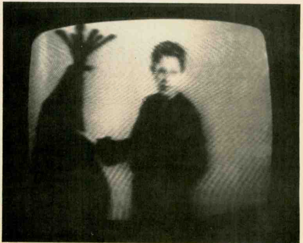
'Herringbone' pattern caused by adjacent channel interference.
