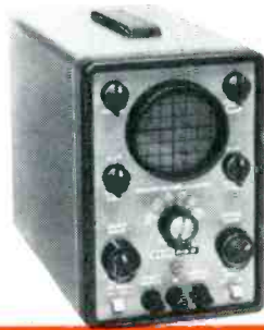
Eico's Model 430 has 3-in. CRT, weighs only 11 lb.
