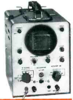
RCA's Model WO-33A has both wideband and narrowband vertical channels.
