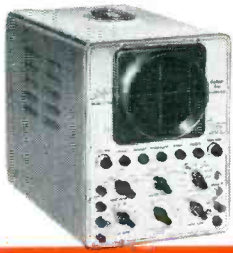
Hickok Model 675A has 20 mv rms/in. sensitivity and 80-nsec rise time.
