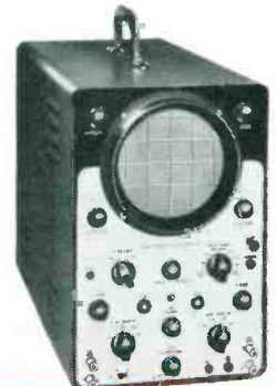
Precision's Model ES150 has 80-nsec rise time and vertical frequency response \pm 3 db 0 to 4.5 Mc.
