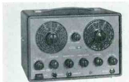
Eico Model 369 features post-injection marker generator.
