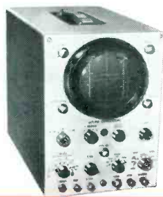
RCA Model WO-91A has vertical sensitivity of 53 mv rms/in. and vertical response \pm 1 db 3 cps to 4.5 Mc.
