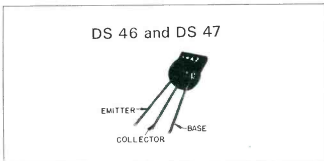
New Delco transistor mount has collector in center.
