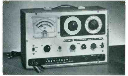
Transistor Radio Analyst is a troubleshooting instrument but checks transistors too.
