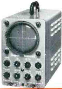
Simpson Model 466's horizontal frequency response is down 3 db at 600 kc.
