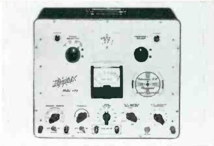
This model has output level meter and three frequency bands.
