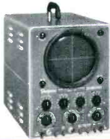
Simpson Model 458 has 7-in. CRT and vertical response \pm 2 db 10 cps to 5 Mc.
