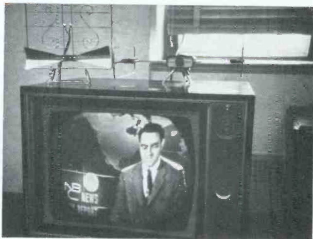
The tube was replaced with good results. The indoor type antennas shown performed well in New York City.
