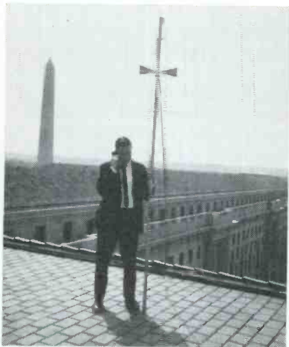
Probing for the best antenna location using an intercom between the receiver position and the antenna.
