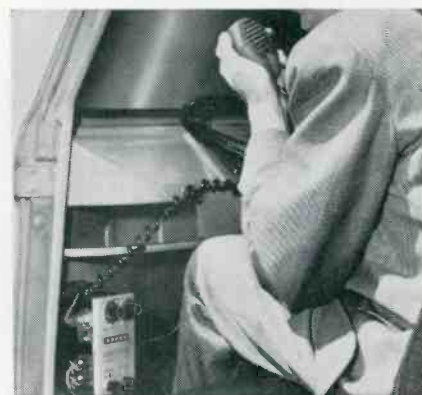
Transistorized mobile 25 w amplifier operates from 12 v battery.
