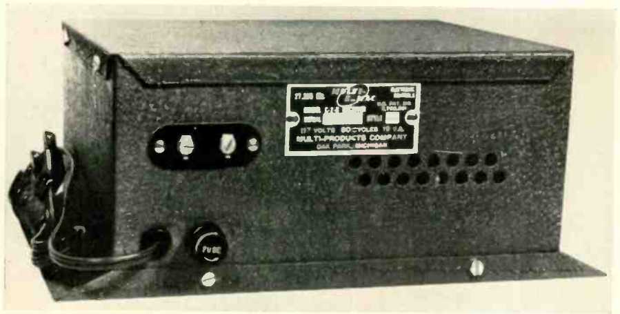
The Multi-Elmac receiver is typical of most tube type garage units. The power consumption is less than 20 w.
