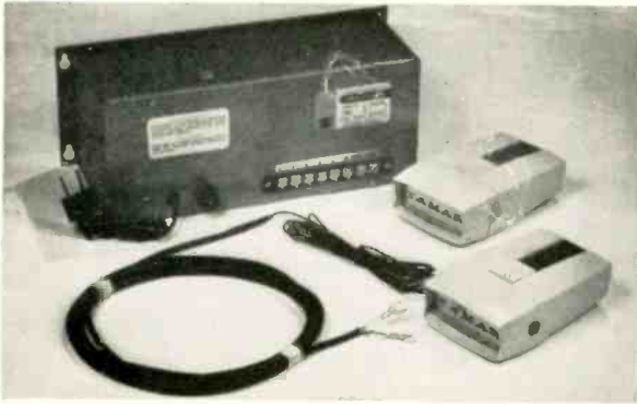
A complete remote control system made by Tamar Electronics Inc., showing two hand-held transmitters. The transmitters have clips for attaching to the sun visor when not in use.
