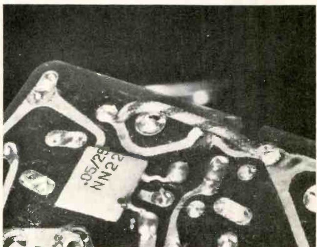
Bridging badly damaged PC wiring with a piece of hook-up wire is usually the best and easiest way to make the repair.
