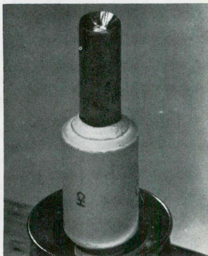
A close-up of modified element after well has been drilled in tip.
