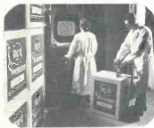
Final checkout. At the end of the production line, just prior to packaging, sample batches of Silverama picture tubes receive a focus check for additional assurance of quality.
