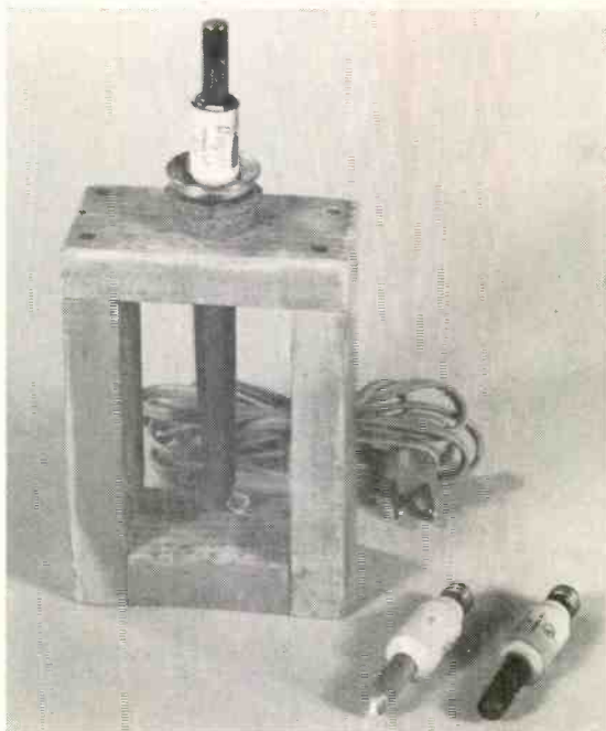
Stand used for holding solder pot. The left element at lower right has a shallow well drilled in its tip.
