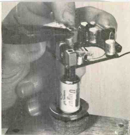
An i-f transformer is easily removed from shirt-pocket radio with solder pot.
