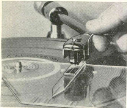
Items like Prestige Products' stylus alignment device can simplify adjustments of various hi-fi set components.
