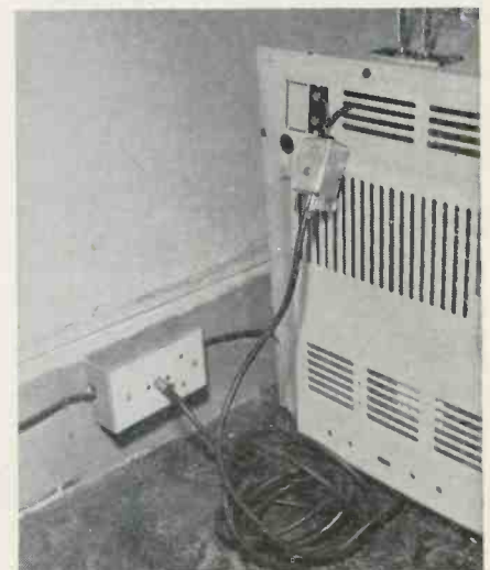
Signal tap-off mounted on wall base & 72 to 300 ohm matching transformer on TV.
