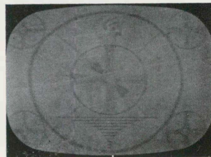
Fig. 6—This dim washed-out picture was caused by a shorted coupling capacitor in set's 1st video i-f amplifier.
