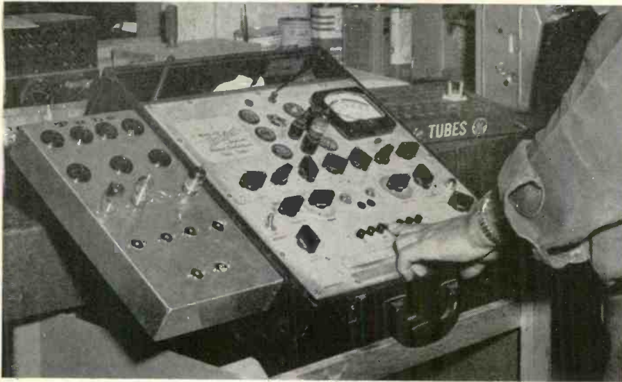
(Top) Tube filament warmer fastened to a commercial tube tester. (Bottom) Wiring diagram of filament warmer illustrates how filament voltages are tapped from the tester.
