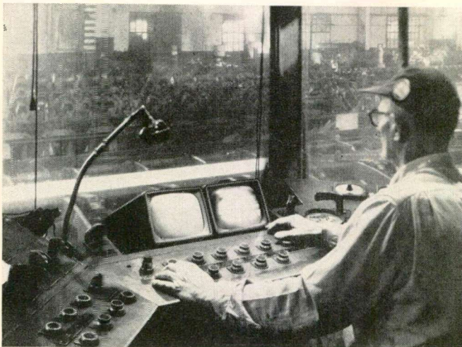
Fig. 3—Operator in control pulpit makes certain steel tubes are properly positioned, using two separate TV monitors.
