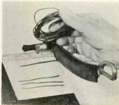
Fig. 2—Hook-up wire can be cut to exact lead length by utilizing a fairly heavy bladed paper trimmer, as shown.
