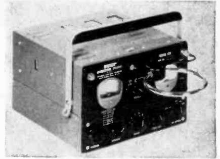
Fig. 2—A professional type noise locator permits rapid location of interference sources.
