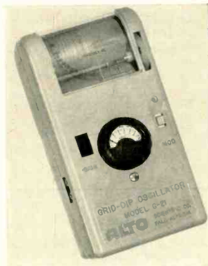
Fig. 3—The grid dip meter shown can be used to check transmitter frequency of parallel resonant circuits without applying power.
