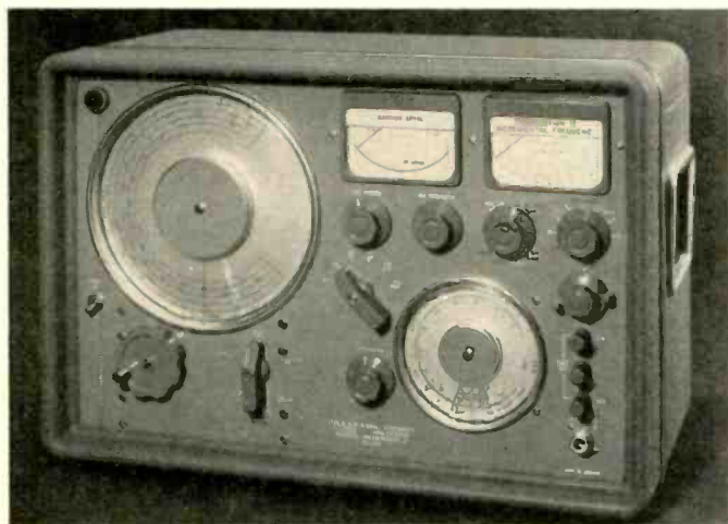
Fig. 1—The illustrated AM/FM signal generator covers frequency range of 10 mc to 470 mc. Calibration is accurate to 0.5%.
