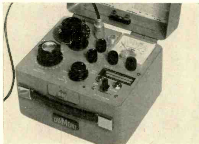
Fig. 2—This transistorized frequency meter is battery-powered for in-the-field mobile communication equipment maintenance.
