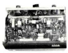
Top view of generator with case removed showing circuit board and components employed in the compact unit.
