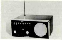
users. It searches at the rate of 12 channels per second, locking on the first active channel. When the transmission ends, the signal search continues. A red light blinks for each channel scanned and the light stays on during a transmission to identify the active channel. Any desired channel may also be manually selected. The radio may be used conventionally or mounted in a vehicle. A 117vac power cord, 12vdc power cord and mounting brackets are furnished. Weigh-
