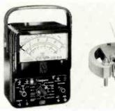
a change in repeatability of less than 0.2%. The taut band movements withstand moderate shock and vibration which cause errors in pivot and jewel instruments. The response of the taut band meters reportedly offers smoother operation and eliminates noticeable overshoot. These Volt-Ohm-Milliammeters come in a broad variety of ranges and accuracies with Add-A-Tester Adapters
