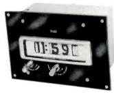
improved appearance opportunities. The clocks are engineered for installation in any equipment or products, rack, console, cabinet and panel; and are designed for convenient economical mounting. Other features include large 5/8in. digits...front panel time reset facility, digits resettable individually. Size: height 3 1/2, width 5 1/2, depth 3 1/4in., weight 3 1/2 lb. Pennwood.
