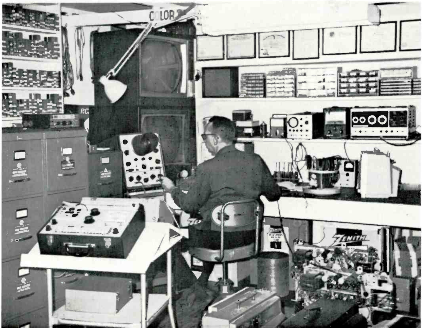
One of the service technicians performs a final check on a color chassis before re-installation.
