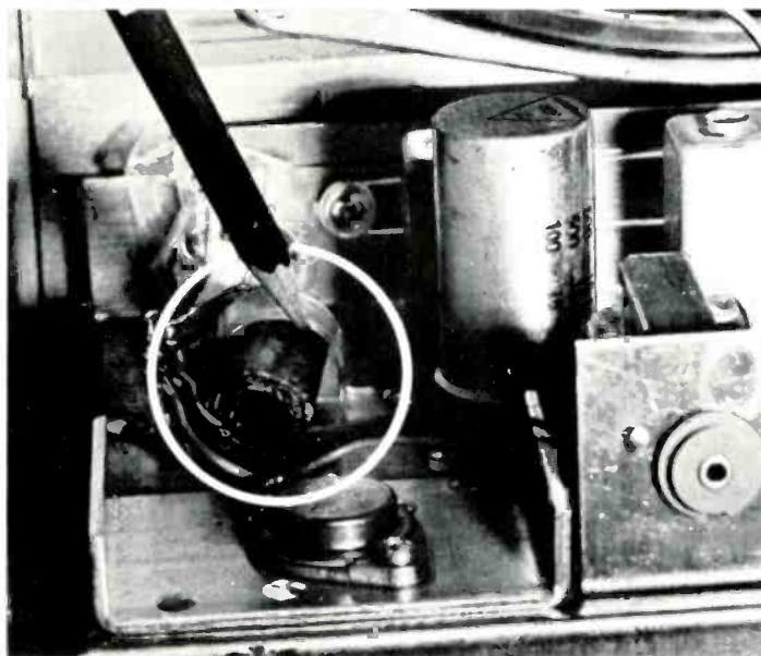
Fig. 2--The choke coil "A" lead is quite often broken by vibration and should be resoldered, then cemented in place with a rubber silicone cement.
