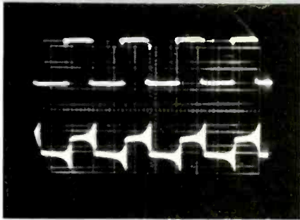
Fig. 2 — Hash (bottom trace) was noted at the collector of the right-channel pre-driver. The signal was good at the base (top trace).
