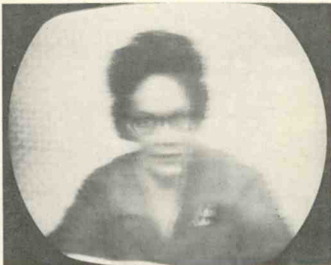
Fig. 8 — This picture was caused by a shorted 21CG8 CRT in a Packard-Bell color set.
