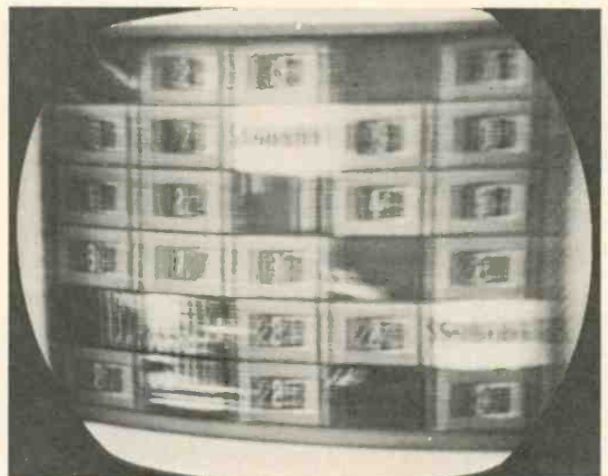
Fig. 6 — Smeary picture caused by shorted delay line.
