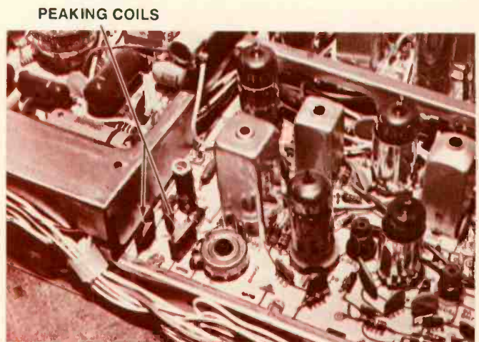
Fig. 4 — Peaking coils in a Sylvania model D-03 chassis. Note the different types. One is wound and enclosed in dipped insulating material. The other is encased in molded plastic and has leads at bottom and top. Some peaking coils have resistors shunted across them with leads protruding at the top.
