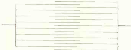
Fig. 3 — Reducing the area of each set of surfaces, adjacent to another set, reduces the capacitance.
