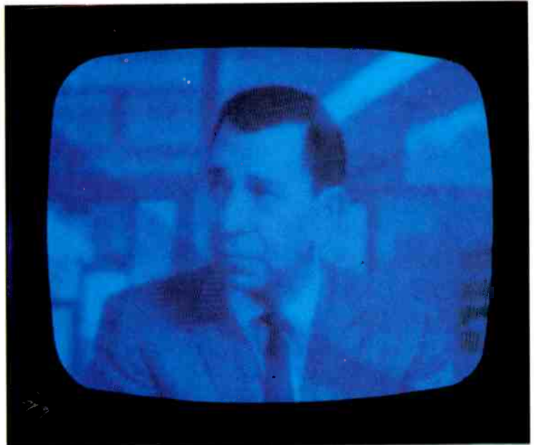
Fig. 4—Blue screen caused by open synchronous detector diode, Y502.
