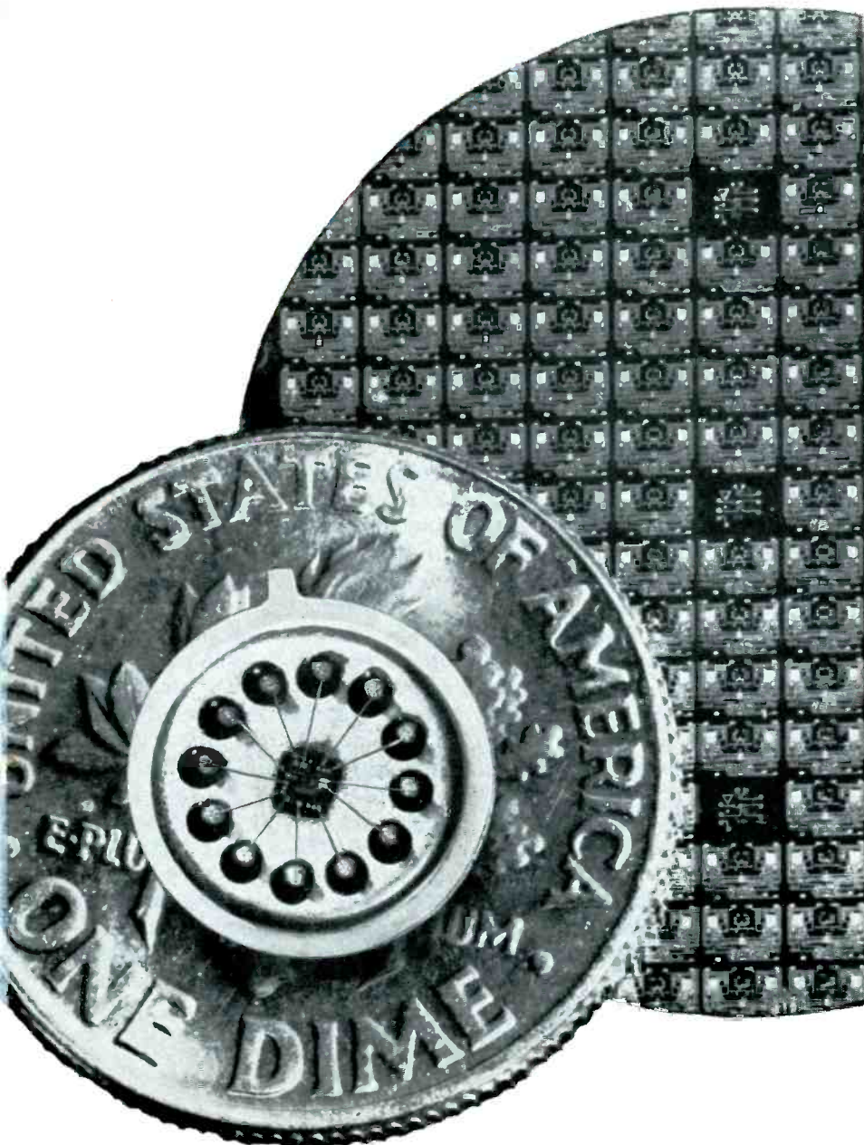
Fig. 1—Approximately 135 usable circuits have been formed on a silicon wafer not much larger than a dime. The relative size of a complete integrated circuit unit is shown on the face of a dime. Courtesy of Motorola.
