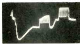
Good duplication of station signal including back porch. If the set won't sync, the set is defective.
