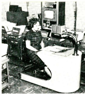
CC-TV "scooter" at the Pioneer Bank & Trust Company, Shreveport, La., moves on tracks in front of the bank's files and sends pictures to monitors at key locations in the main and branch banks. Teller, bank official, or customer sees requested information on one of the many monitors used throughout the system.
