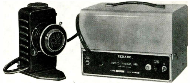
Fig. 4—This 150-w xenon lamp is used for microscope illumination and has an accessory which briefly pulses the lamp to a higher level for making photomicrographic exposures. Most of its circuitry is shown in Fig. 1.
