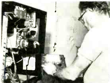
Fig. 3—Discharge high voltage lead and disconnect from CRT.
