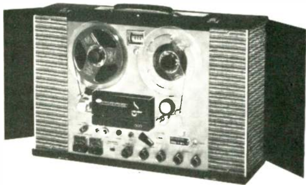
"Packaged" stereo recorders are appearing in increasing numbers. Concertone's model 510 is an example of a complete high quality unit.
