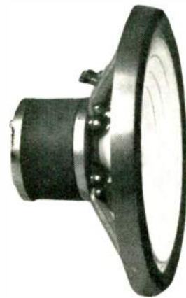
Hartley Products' loudspeaker uses a patented system called Magnetic Suspension. In place of "spider" cone centering mechanisms, the magnet's force is employed to center the cone. Response is 20 to 20,000 cps.
