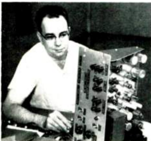
Advanced Engineering. Scott begins in the laboratory where the Advanced Development Team pioneered Wide-Band Design and "Time-Switching" multiplex circuitry. Chief Engineer Daniel Von Recklinghausen is shown here with the original model of the world's first commercial FM Stereo signal generator, which is used by manufacturers throughout the world.
