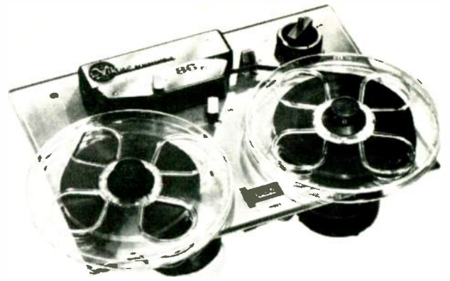
Viking playback tape deck is designed for use in custom installations or as an integral part of packaged recorders.
