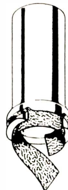
Fig. 3—Standard tube shield used for r-f injection. A small amount of masking tape is wrapped around it's base to prevent grounding.
