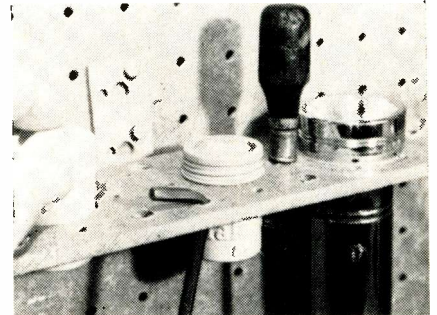
A pegboard shelf holds flashlight, tools and small parts in 35 mm film cans.
