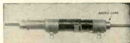
Fig. 3—Extra core increases inductance
