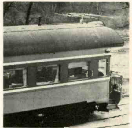
Taco Trapper antenna atop railroad car.
