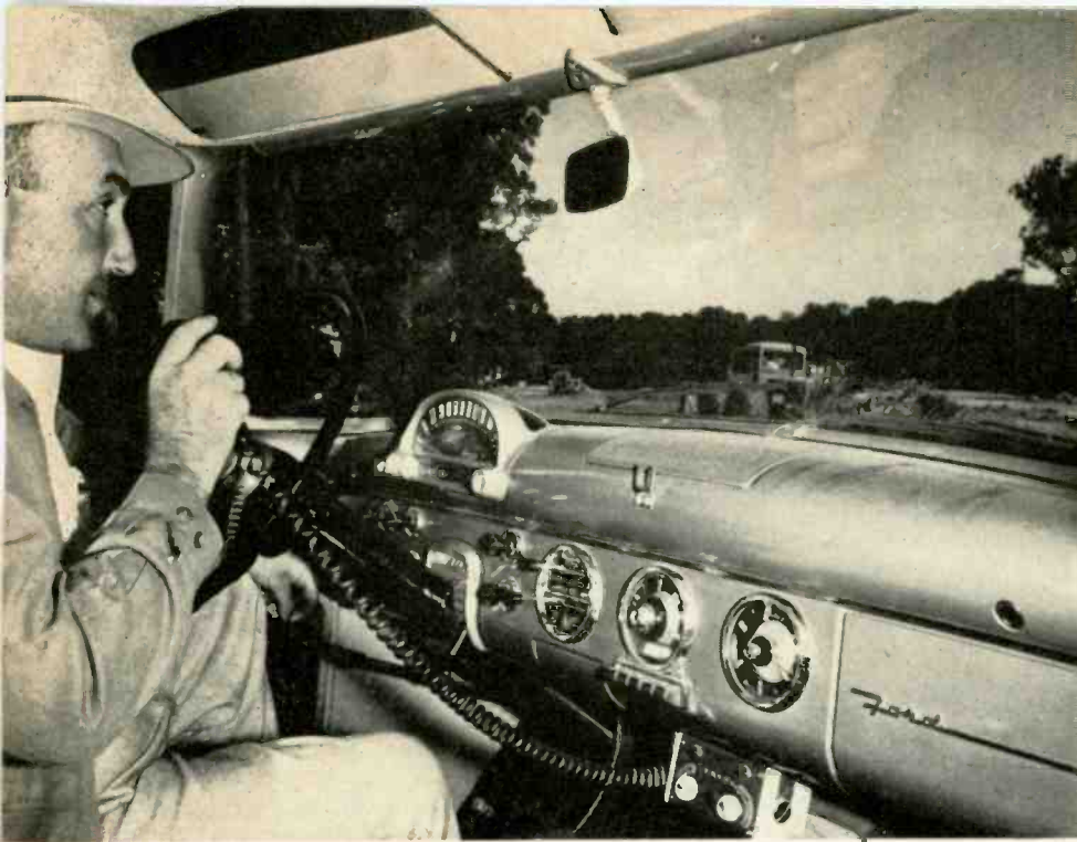
Typical mounting of the control head and the speaker for a trunk-mount installation.
