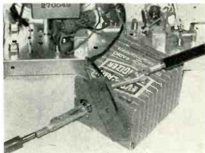
Fig. 2—For battery type shown, unclip one end of battery lead for current measurement.
