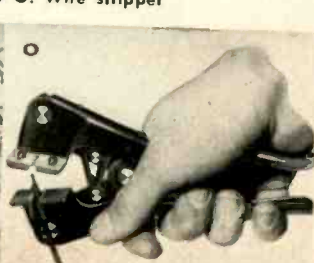
K. Roll-away service bench L. Wall-mounting transparent rack M. Printed circuit kit N. Probe O. Wire stripper
