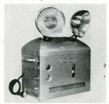
tional Fire Code and is UL-approved. The glass jar battery can deliver 91% of rated capacity after 30 minutes of actual use. Features include external switches for testing; switches to control the battery charger, and to disconnect lampheads for servicing; red pilot light to indicate when battery is on high charge; an amber light to indicate readiness for service; visible discolor hydrometer. Carpenter Mfg. Co., Boston 45, Somerville, Mass.—TECHNICIAN
