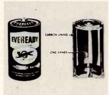
D99 is made to sell for a price slightly higher than standard general-purpose batteries. The zinc electrode of the cell is on the inside, while the carbon is on the outside. This reverses the design of standard flash batteries. As a result, consumption of zinc during use goes on inside the cell. Manufacturer guarantees free replacement of flashlight, if it is damaged by the use of this long-life cell. National Carbon Co., 30 E. 42nd St., New York 17, N.Y.—TECHNICIAN
