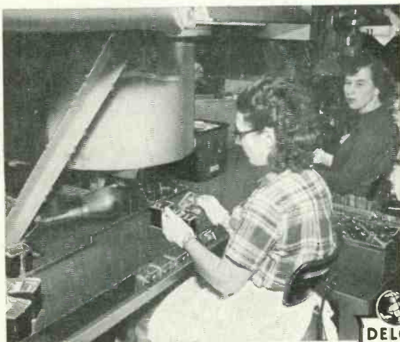
Potting power transformers. The transformer can is filled with an asphalt compound which helps to protect the transformer and transfer heat from the transformer to the can for better heat dissipation.
