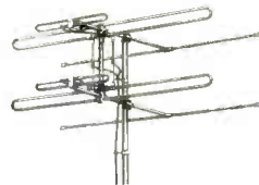
Model 114-322 INLINE Stacked Array includes two INLINE bays, connecting rods, two mast clamps, two 5-foot mast sections, guy ring, stand-off insulator and 100 feet of Twin-Lead.
