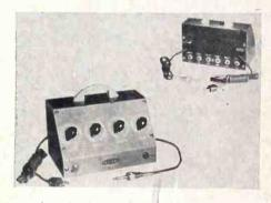
unit has four controls for a wide range of blending on its four channels. The six inputs include four mike and two phono. Frequency response is 20-20,000 cycles, hum level is said to be extremely low. Pentron Corp., 221 E. Cullerton St., Chicago 16, III.—RADIO & TELEVISION RETAILING.
