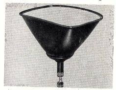
19 inches. (The 16AP4 was 221/4 inches long.) The tube incorporates a frosted filter-glass face plate for improved viewing, said to eliminate annoying room reflections as well as halation and reflection within the faceplate itself. A single-field ion trap is employed, as well as magnetic deflection and focus. Tube Department, RCA Victor, Harrison, N. J.—RADIO & TELEVISION RETAIL-ING
