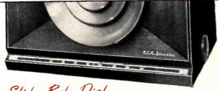
Slide-Rule Dial Point out to your customers how the engraved calibrations on molded plastic, edge-lighted with two pilot lights, make an attractive easy-to-read dial arrangement.
