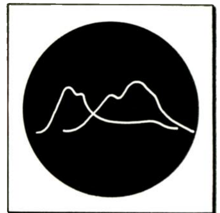
Fig. 2—Improperly phased response curve. Adjust phasing control of sweep generator or scope to bring two curves to maximum overlap.
