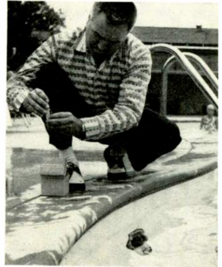
Fig. 1—Measuring PH factor with a water test kit to avoid damage to a submerged speaker.
