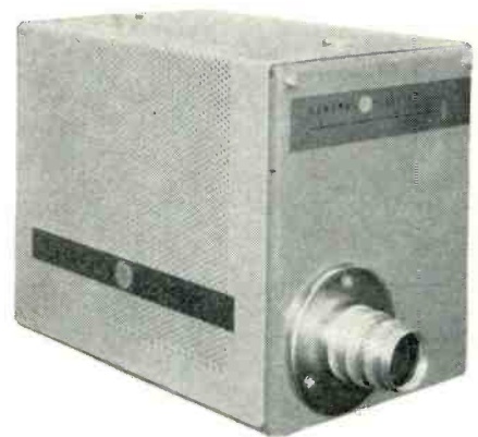
Fig. 2—Camera contains a vidicon CRT, video preamplifier and a blanking amplifier.
