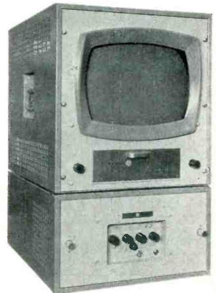
Fig. 4—Control unit under the master monitor contains sync, sweep and video chassis. Corrected for phase, clamped, additional blanking added, and then fed to the monitor through a level control. An
