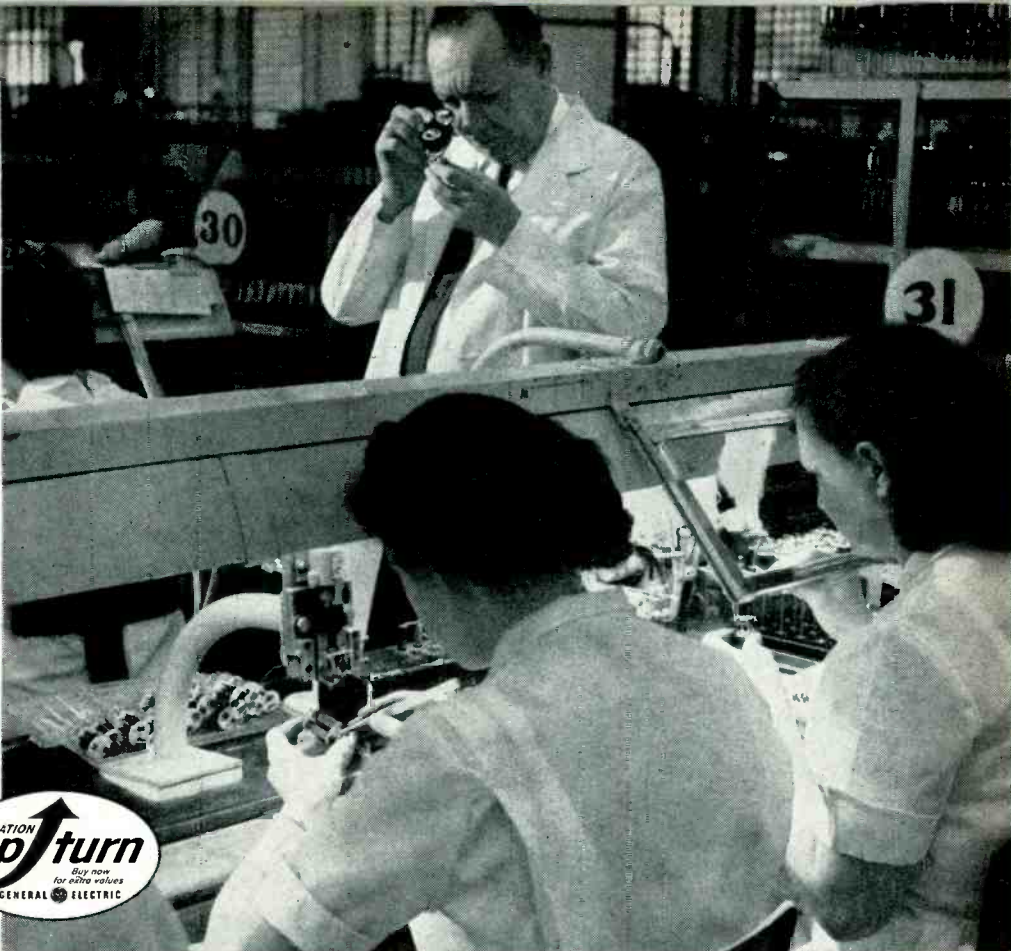
ABOVE: LINT AND DUST ARE BANNED during "Snow White" assembly of General Electric receiving tubes, in order to reduce the possibility of short-circuits. G-E workers and supervisors wear lint-free garments; air is filtered and conditioned; floors are kept immaculately clean.
