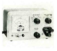
30 volts output. A line voltage change of  $\pm 10\%$  causes output change of less than  $\pm 0.2\%$  or  $\pm 15$  mv, whichever is greater. The output voltage temperature coefficient is approximately 0.2% per °C, 24°C to 50°C. Hewlett-Packard Co., 275 Page Mill Rd., Palo Alto, Calif. (ELECTRONIC TECHNICIAN 5-30)
