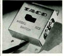
sign permits mounting at rear of receiver cabinet. The 823 is designed for switching between two antennas at the receiver. It is also recommended for use in antenna switching, for switching antenna between two receivers or in the case of hi-fi systems, for switching loudspeakers. Technical Appliance Corp., Sherburne, N. Y. (ELECTRONIC TECHNICIAN 5-35)
