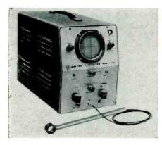
circuit and display its waveform on the CRT. Audio circuits may be monitored aurally as well as visually. It will test tubes in their crcuits; and may be used as a field strength indicator, an oscilloscope, a waveform analyzer, and as chassis-top signal tracer. Kingston Electronic Corp., Medfield, Mas (ELECTRONIC TECHNICIAN 5-20) Mass.
