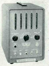
Fig. 9—Commercial counter with plug-in elements, provide speed and precise indication.
