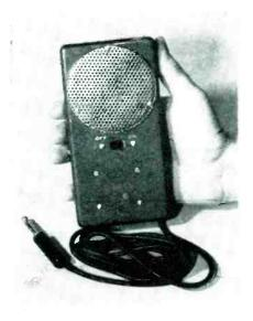
A small but powerful power amplifier and speaker utilizes 3 transistors. Its self-contained batteries will operate for over 700 hours. It is a practical and easily-handled accessory for any earphone-style tape or wire recorder, radio receiver, or amplifier. The unit is used in place of an earphone.
