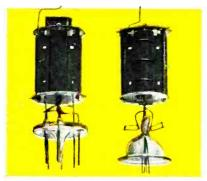
Notice how much more rugged the Sylvania wafer stem mount looks (left). That's because the wafer stem results in shorter construction with more points of support and heavier, sturdier leads.
