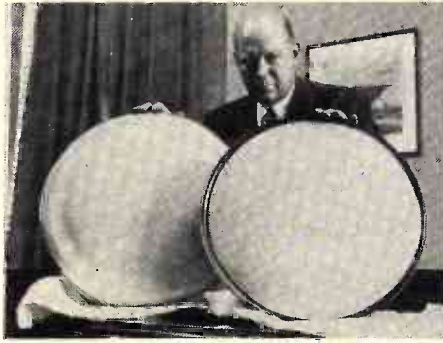
Dr. Allen B. Du Mont, president, Allen B. Du Mont Laboratories, Inc., compares the old 20" cathode-ray tube (left) with new short-necked metal 19" Du Mont television tube, introduced in the firm's Bradford console model. The new tube is only 21½" long.
