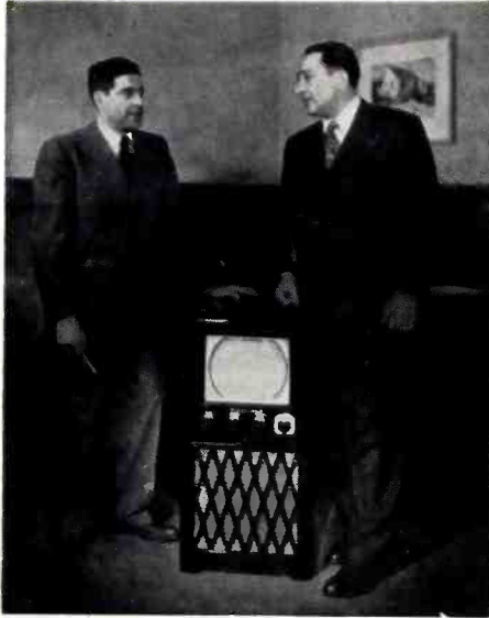
The Siragusa brothers, left, Dom, president of Molded Products Corp., and Ross, right, president of Admiral Corp., discuss Admiral's new 24 tube TV plastic console. The set has a 10-inch picture screen, and list price is $249.95. The cabinet is Bakelite phenolic and weighs 35 lbs.
