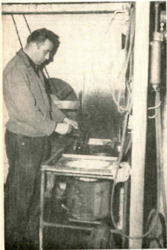
Paint spray booth has sinks for washing motor, other parts. Fumes are expelled at rear of booth. Trade-ins are put in top condition.
