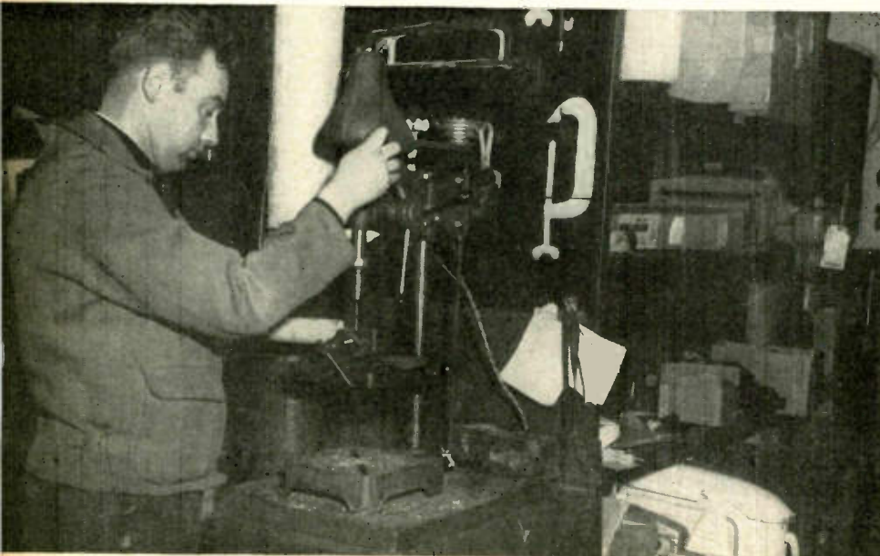
Below, both large and small drill presses are in regular use at Beckley's. Note neat placement of C-clamps, hacksaw, drill press parts on outline panel on wall.
