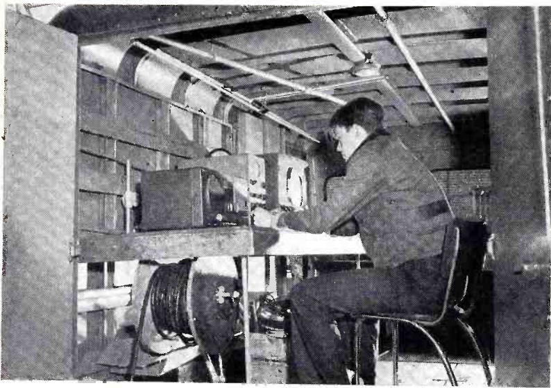
Inside the truck: all-wave receiver, 'scope, monitor TV set, and reel of wire to feed in 110-AC from customer's home.
