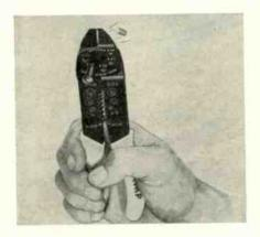
pliers-like tool. Holes are provided for different sizes of screws and wire. Handles are shockproof plastic. Aircraft-Marine Products Inc., 1523 North 4th St., Harrisburg, Penna.—RA-DIO & TELEVISION RETAILING
