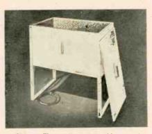
sterilizing. The unit is portable, requires neither special wiring or pressure water system. May be used also for steam or dry sterilizing, and for washing equipment or clothing. Heat is supplied by "life-belt" element attached to outside of the tank. Tank interior has smooth, galvanized surface. Designed to heat small quantities of water quickly, twenty gallons in a few hours. Equipped with temperature control knob. Clark Div., McGraw Electric Co., Chicago, Ill.—RADIO & TELEVISION RETAILING
