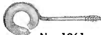
No. 1961 Split Bridge Ring Insulated Screw Eye, Overall length 3-5/8", 5/8" insulator hole, 1/4" diagonal slot.
