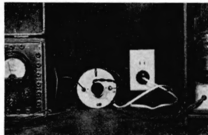
Outlet box is permanently connected to wall receptacle. To eliminate meter and shunt, use a jumper with pin jacks at either end.
