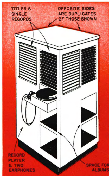
▲ Wm. D. Barrow (see story p. 64) designed this unique display-storage-record player piece.
