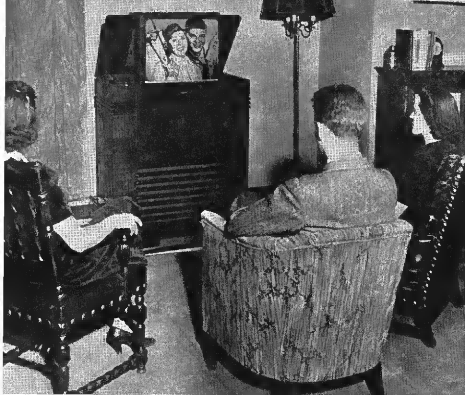
RCA—Latest home design produces picture on translucent screen 13½ by 18 inches overall. Screen is retractable. Kinescope picture is projected through lens to mirror on underside of cabinet's lid and, from here, is reflected to viewing screen
