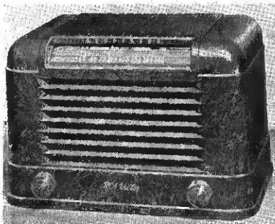
RCA PLASTIC TABLE-TYPE radio known as the "Foreign Correspondent" covers foreign and broadcast bands. A 5-tube superhet with ac-dc operation tunes from 8600 to 12,000 kc and spreads the popular 25 and 31-meter short-wave bands. RCA Mfg. Co., Camden, N. J.
