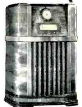
MODEL 103CK2, "Self-Tuning" Motorola; Automatically Tunes Station after Station all day long; 10 Tubes including Rectifier; 3 Gang; 6 Push Buttons; 3 Bands; 12" Speaker; Semi-Rotable "Aero-Vane" Loop; Magnificent Walnut Veneer Cabinet; Television, F.M. and Phono Connection.
