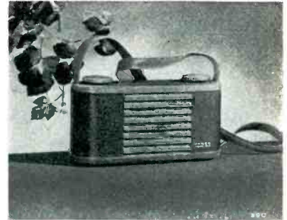
CANDID PORTABLE—Portable Model 89C radio. Hangs on shoulder like cameracase. Weighs five pounds, measures 5 x 10 x 4 inches. Special braided aerial wound inside shoulder strap. Extremely small battery block is self contained.
