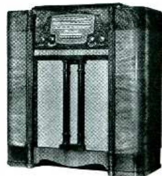
MODEL AC-91 . . . A lowboy console exemplifying the rare artistry of Farnsworth Radios. Chassis Specifications . . . 10-tube superheterodyne; Flo-Lite dial; three wave bands; shielded rotatable loop antenna; continuously variable tone control; push-button tuning; 12" electro-dynamic speaker; beam power output; phonograph and TELEVISION-sound connection. Cabinet dimensions: Height, 35 \frac{1}{4} "; Width, 32 \frac{1}{8} "; Depth, 13".
