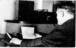
COMPACT CONTROL—This new and novel unit with a 45-degree angle case comprises speaker, mike and switch. An external amplifier is used. (Sound Systems, Inc., Cleveland)
