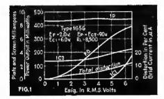
tube. For lowest distortion with a chosen plate load resistor the bias should be selected so that just enough grid potential swing is secured to produce the desired output without permitting the grid potential to reach the grid current region.
