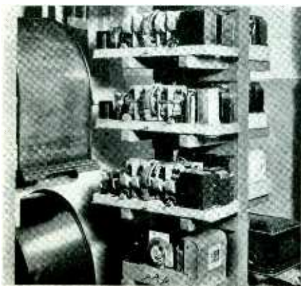
Two 1 in. by 2 in. wooden uprights with "T" cross-arms form a convenient rack for chassis in the Beaucaire & Mitchell (Rochester) shop, taking up little floor space
