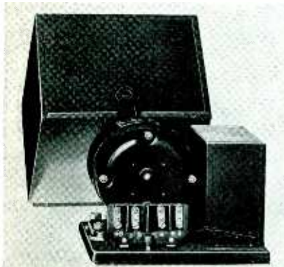
Dynamotor. (Emerson) Filter designed to eliminate commutation ripple is in the square "can"
