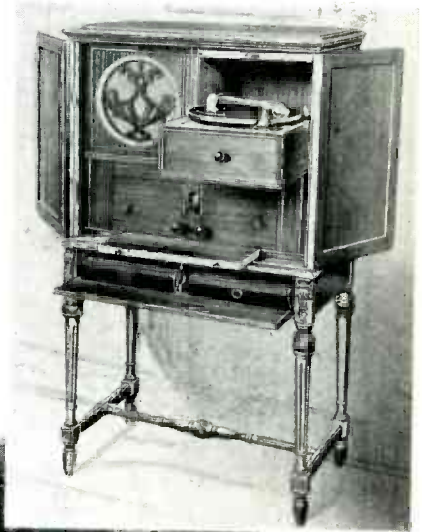
THE UNION ELECTRICALLY COMPLETED. Electric pick-up and the amplification of recorded music via the audio amplifier of a radio receiver was developed in 1927. All-American's model 88, equipped with a.c. tubes, is representative. It sold for $425.
