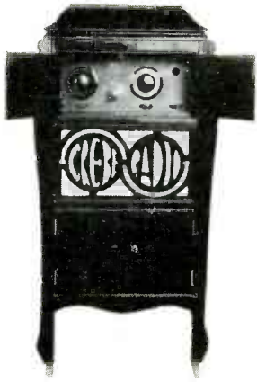
AN EARLY "COMPANIONATE" MARRIAGE. Grebe's "Radiotone," introduced in 1922 at $310 list, was one of the first combinations. The phonograph was of the old mechanical reproducing type with a horn speaker. The radio was a CR-5, tuning from 150 to 3,000 meters.
